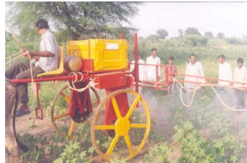
Training cum demonstration of bullock drawn sprayer in cotton
