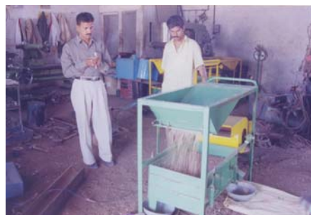
Power operated grain cleaner mfd by M/s Ajay Ind, Amravti & it's testing
