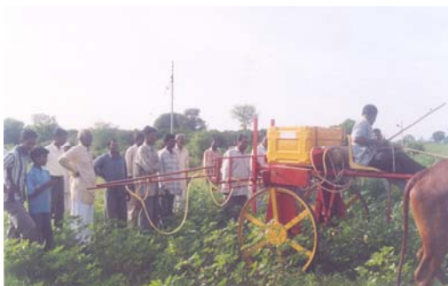
Training cum demonstration of bullock drawn sprayer in cotton
