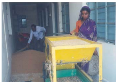
Demonstration on Power operated grain cleaner
